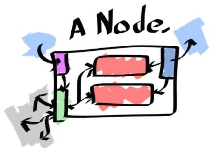
In a Lighthouse setup, no node's application code is aware of the existence of other nodes, they talk to a local port handled by an instance of the load balancer which in turn routes traffic among the various known other nodes.
