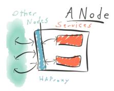
In a Lighthouse setup, no node's application code is aware of the existence of other nodes, they talk to a local port handled by an instance of the load balancer which in turn routes traffic among the various known other nodes.
